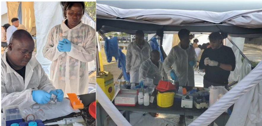
Images 6. Syringe filtration of refrigerated samples collected 6 September — extraction of nucleic acids, NA, from the filters, followed by preservation of the filters for qPCR analysis on day 3.
