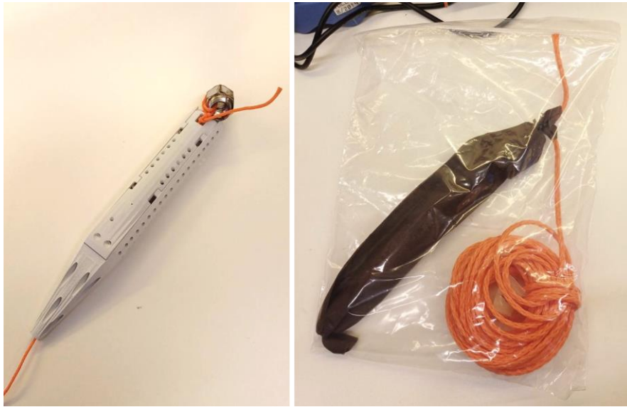
Figure 3. Fully assembled torpedo sampler with weight (left) and additional wrapping with shade cloth (right). Photos: THL.
