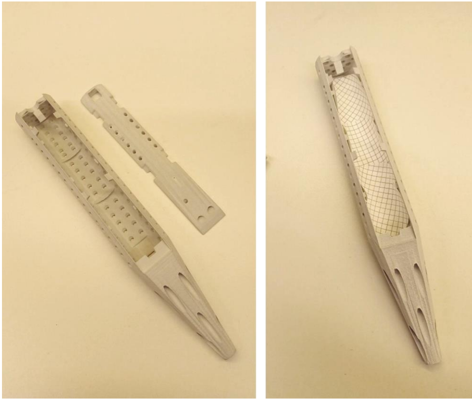
Figure 2. Torpedo-style passive sampler empty (left) and with 0.45 \mu\text{m} membranes inside (right). Photos: THL.
