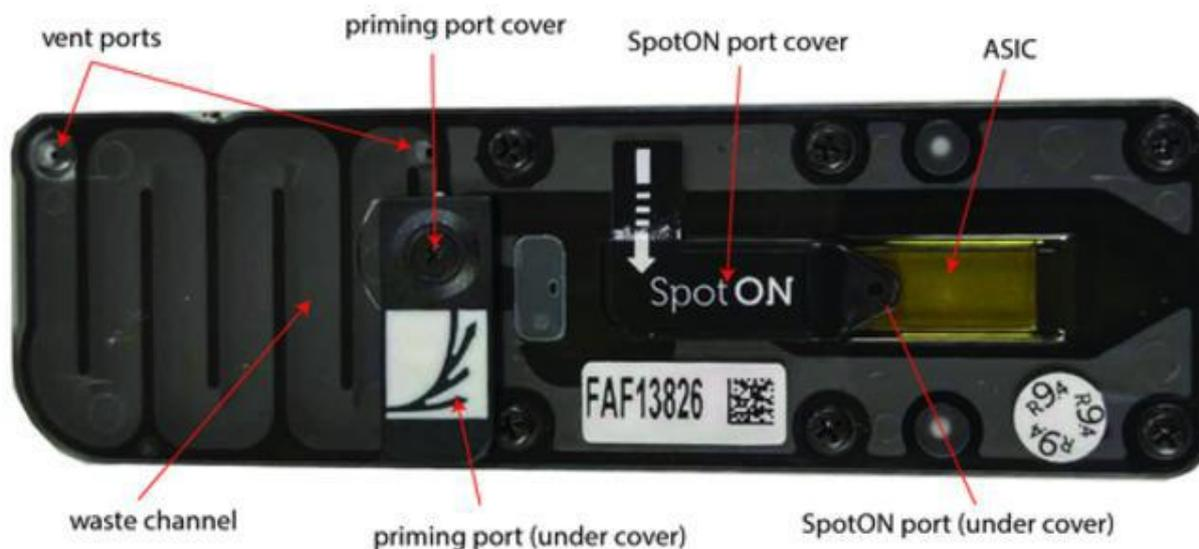
Figure 2. Diagram of an ONT flow cell and the important features. Image reproduced from [Street Science Community](#).
